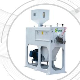
Silky Master Jumbo machines are the latest generation machines that give best quality polishing to rice and give a silky smooth finish to the rice grain. A special device provided with spray gun to get mist form with compressed air and water, it gives superior quality of smooth and silky rice.
