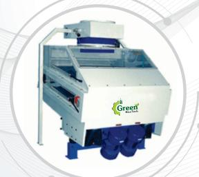
The machine is designed to clean impurities like dust and paddy size impurities in the paddy. This machine functions effectively when the paddy is already precleaned.
